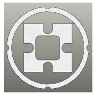
The StrainCell owes its repeatable, stable, and high-accuracy readings to its small and circular design. The sensing frame is specially designed to expand and contract with the metal to which it is attached. Since the sensor is exposed to the same environmental conditions as the structure, the sensor virtually eliminates all the measurement errors by expanding and contracting in every direction, measuring strain in every direction.
